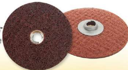
QUICKLOCK "SPINNER" 4 1/2" & 5" DIAMETER (TYPE S UNDERSIDE MOUNT WITH 5/8"-11 SCREW-ON LOCKING STYLE)
